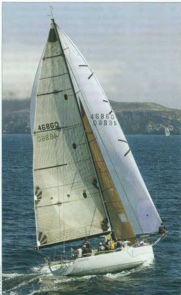
Left —Locomotion is a 45' (13.7m) ULDB, with a D/L of 80, metal fin, torpedo keel, and carbon/E-glass/Kevlar vacuum-bagged hull that circuitously led to development of the TP52 class ( above ) for Los Angeles to Hawaii Transpacs and grand prix buoy racing.
